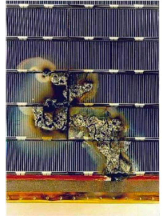
Surface discharge damage to a solar array Ferguson, 2018
