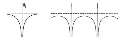
**Figure 3.6.** Schematic depiction of the electrostatic potential of an isolated ion (left) and the superposition of the potentials of neighbouring ions (right). Figure reproduced from KIPPENHANHN & WEIGERT.
