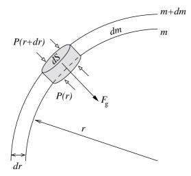
**Figure 2.1.** Mass shell inside a spherically symmetric star, at radius *r* and with thickness d*r*. The mass of the shell is  $dm = 4\pi r^2 \rho dr$ . The pressure and the gravitational force acting on a cylindrical mass element are also indicated.
